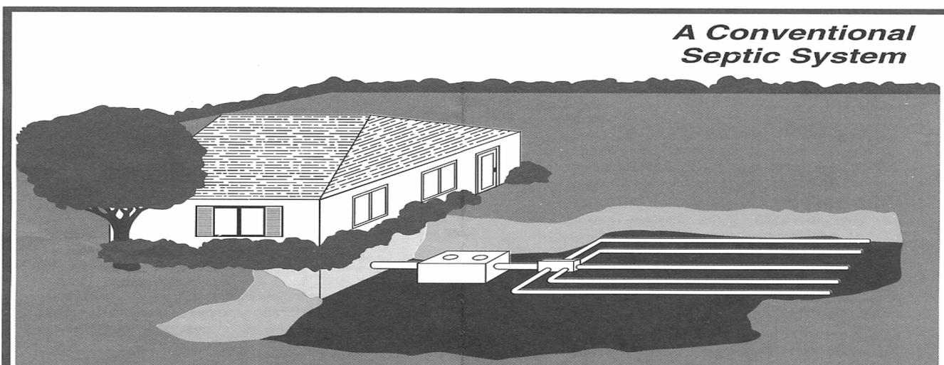
*A **septic system** consists of a **septic tank**, a **distribution box** and a **drainfield**, all connected by pipes, called **conveyance lines**.*
